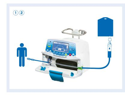
① Open the pump door by lifting the door lever.
